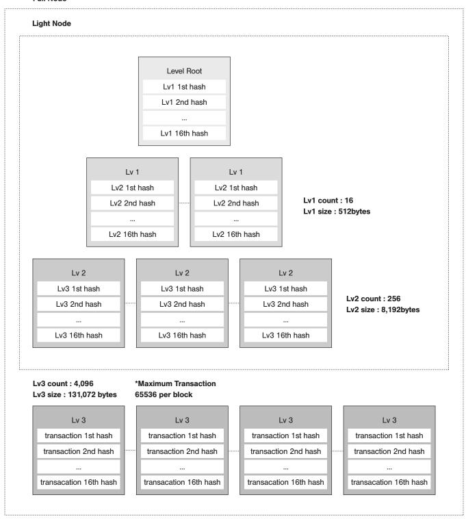
MEVerse employs LEVEL Tree method, clustering 16 blocks as one unit to hash and hash that unit into 16 parts. This is a much more efficient system, making a tree where the hash process of the transaction is simplified, and each level has 16 subunits.
