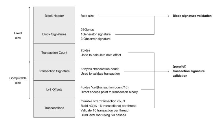
Serialization of the next block is designed to expedite verification of blocks in parallel, with the following structure:
